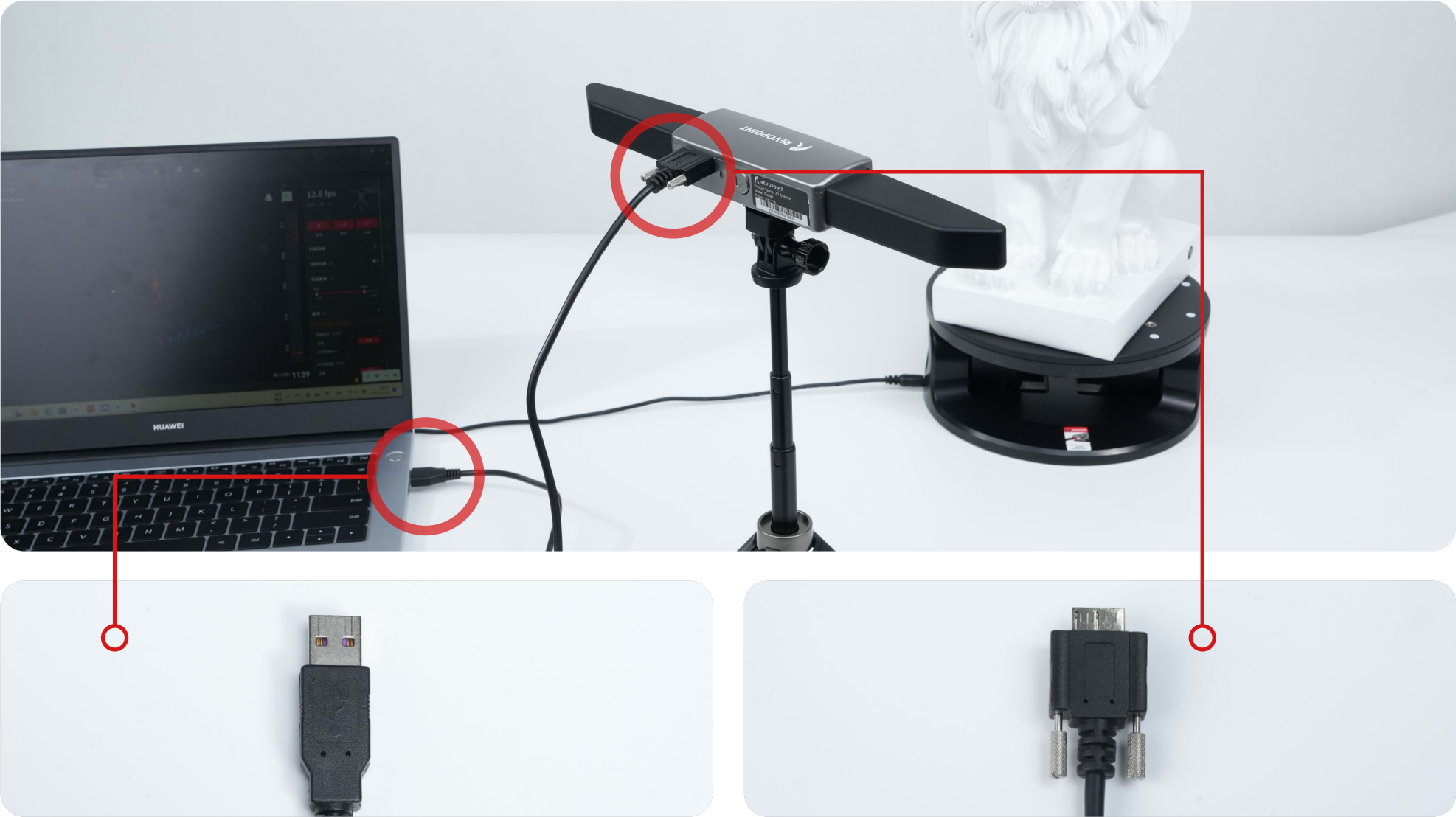
Plug into the PC's USB 3.0 port.
