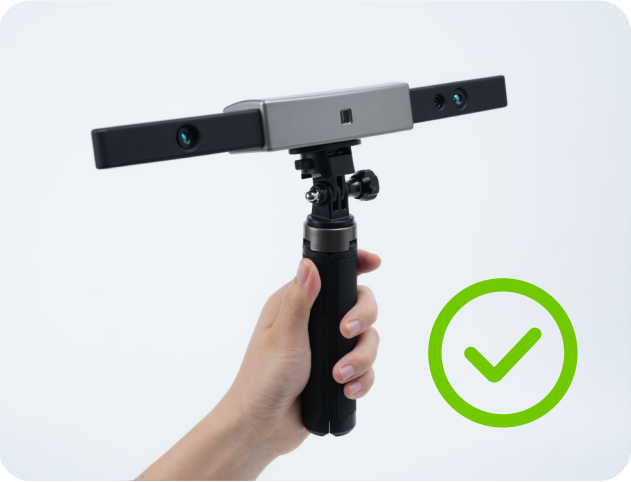
Image 2: Hold the tripod for handheld scanning.
