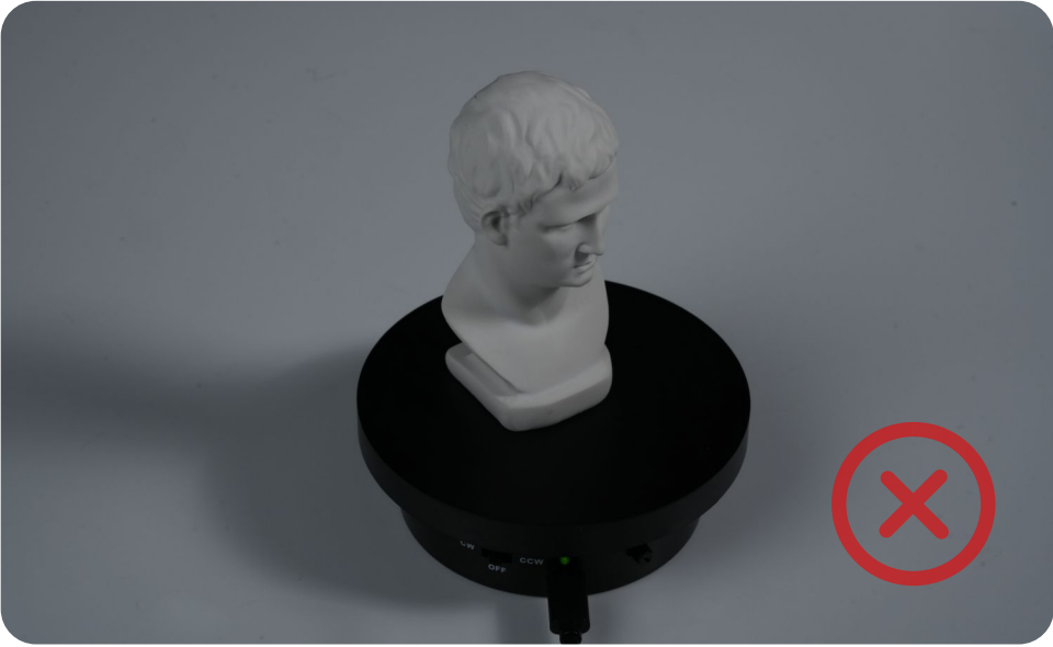
Incorrect Color Scans - Dim lighting conditions are bad for color scanning.
