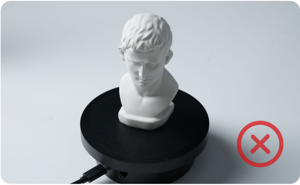
Incorrect Color Scans - Uneven illumination will affect texture mapping.
