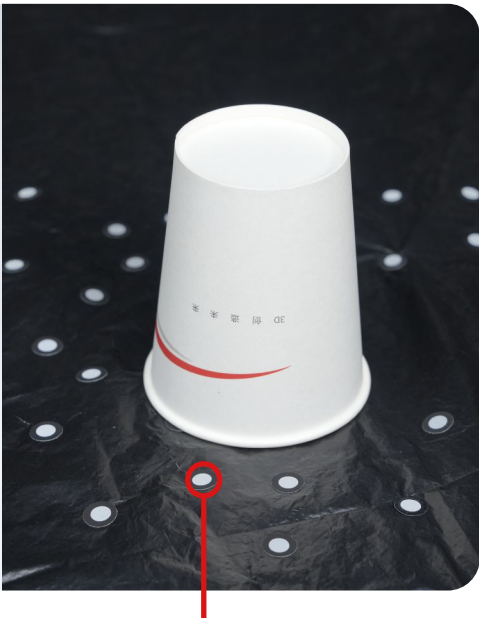
Stick the marker dots around the cup
