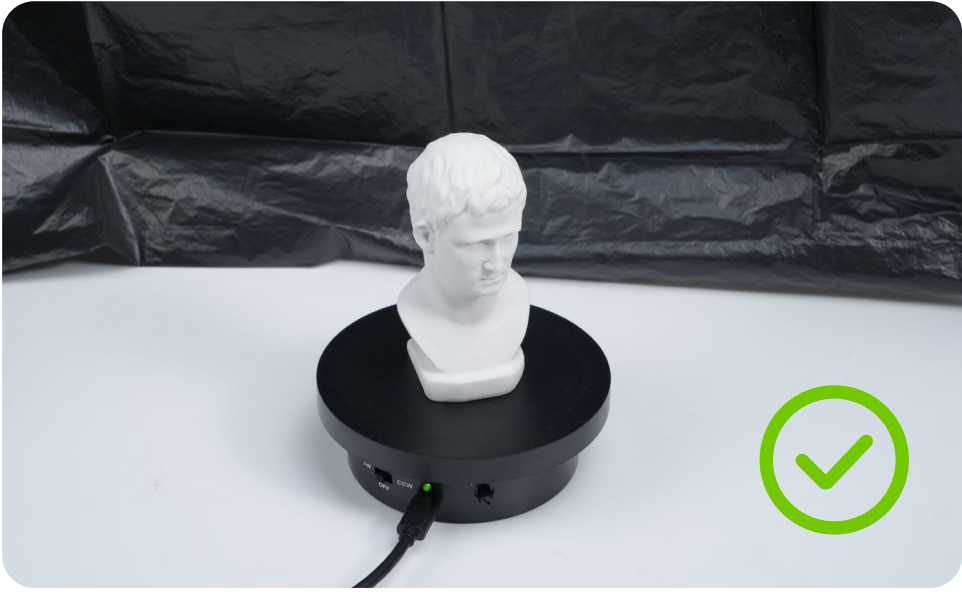
Using a Black Sheet as the background and ensuring consistent and even illumination.
