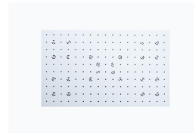
Calibration Board Used to calibrate the MetroX 3D scanner.
